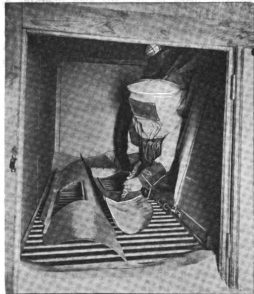
New sand-blast (inside). Operator stands outside the little cage and works inside it
